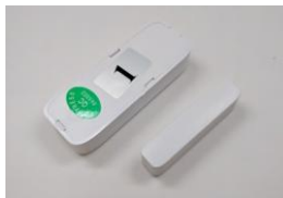
A door/window contact sensor with a #1 sticker.
